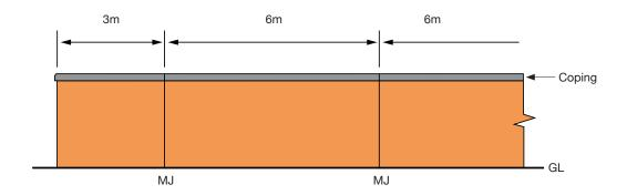
Fig. 4 Parapet wall
