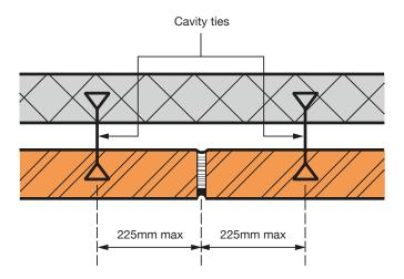
Fig. 13 Movement joint with sleeve debonding tie
