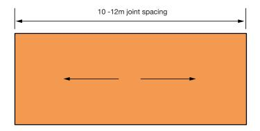
Joint spacing at external returns should be based on being continuous around the corner.
