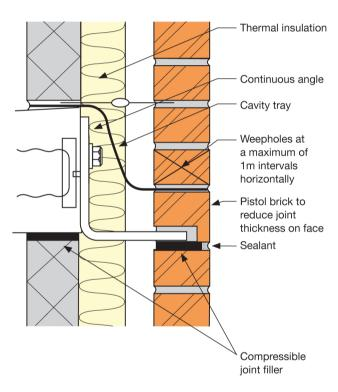
It is common practice to incorporate support at every second storey so providing the opportunity to locate movement joints of reduced thickness.
