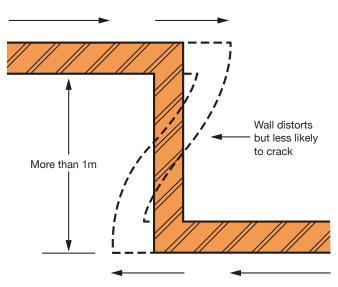
Fig. 9 Alternative arrangement using compression joints at some distance from the corner
