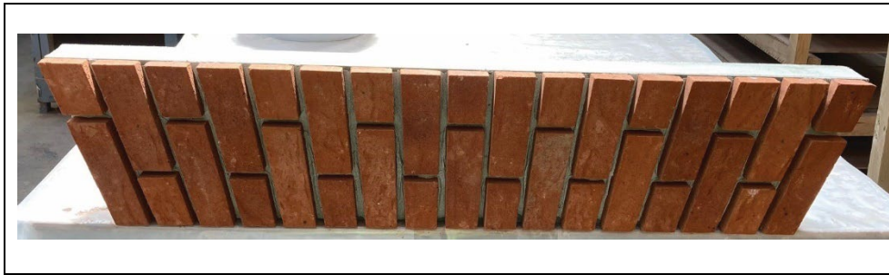
Figure 1 Lightweight Brick Clad Insulated Panel
